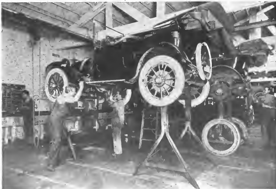
Service racks used by Harold L. Arnold, Los Angeles dealer, to eliminate garage pits
